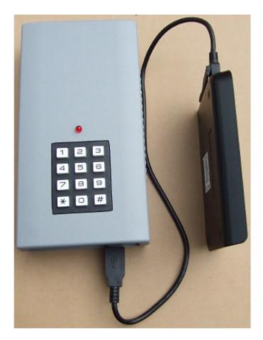
This simple server consist of the MPT4 sound card placed in a standard 100 x 190 mm box and a 320GB portable USB hard drive. The power to the hard drive is supplied via USB connection.
