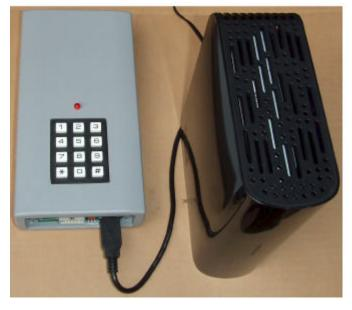
This server consist of the MPT4 sound card placed in a standard 100 x 190 mm box and 1TB external USB hard drive. The 12V power to the hard drive is supplied separately.
